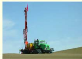
WTC5150 auger drill
